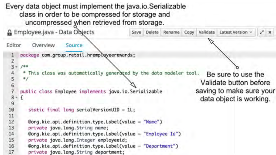
Figure 3.15 The Source editor's the tab that provides a developer view of the actual Java source code that makes up your Employee data object.
