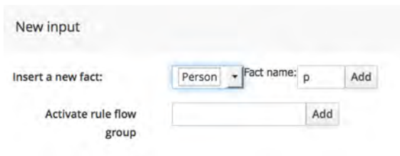
Figure 4.19 Inserting a new Person fact with the name 'p' to allow you to reference it later in the test scenario.
